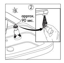
**To clean the filters:** Turn the water off at the stops.
